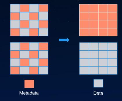
Different types of data synchronously executed in the controller and SSD disk are stored separately
